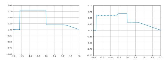
Note that Roe's scheme on the left does not take into account the shocks that Godunov's scheme does, on the right. This would be a result of the piecewise nature of the flux functions with Godunov.
